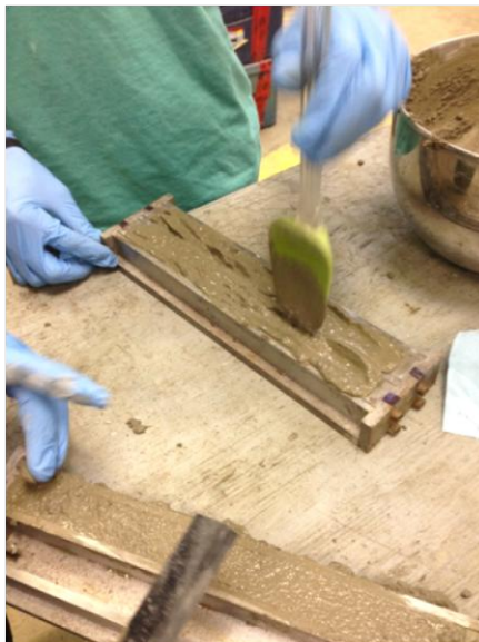
Figure 6: Mortar Bar Test Mould
