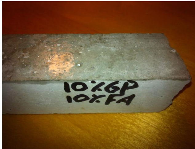
Figure 22: 10GP/10FA Mortar Bar. No Signs of Expansion.
