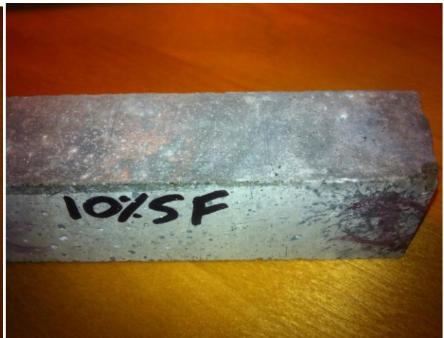
Figure 18: 25FA Mortar Bar. No Signs of Expansion. Figure 19: 10SF Mortar Bar. No Signs of Expansion.
