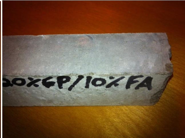
Figure 23: 20GP/10FA Mortar Bar. No Signs of Expansion.
