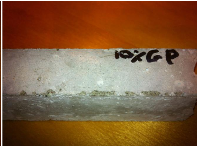
Figure 21: 10GP Mortar Bar. Expansion Cracks Visible.
