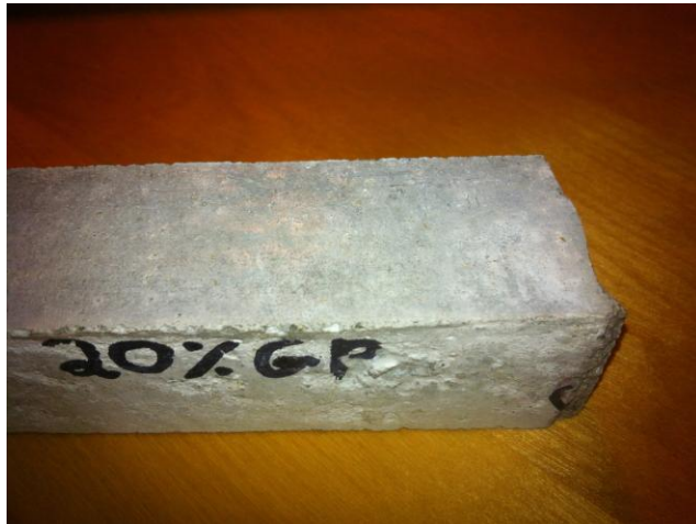
Figure 20: 20GP Mortar Bar. No Signs of Expansion.
