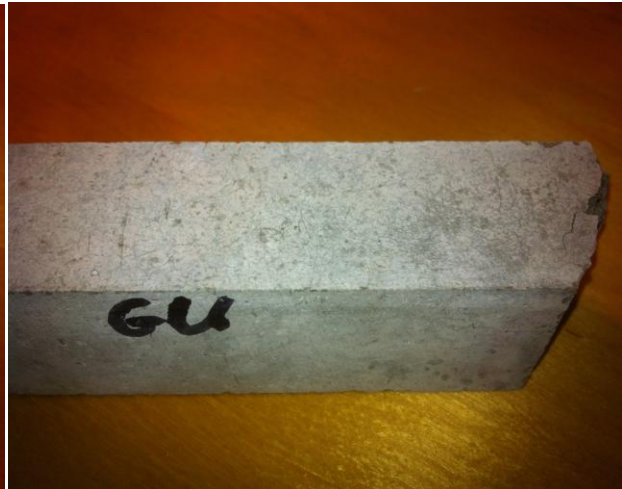
Figure 16: TerC3 Mortar Bar. No Signs of Expansion. Figure 17: GU Mortar Bar. Expansion Cracks Visible.
