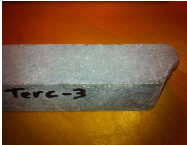
Figure 16: TerC3 Mortar Bar. No Signs of Expansion. Figure 17: GU Mortar Bar. Expansion Cracks Visible.
