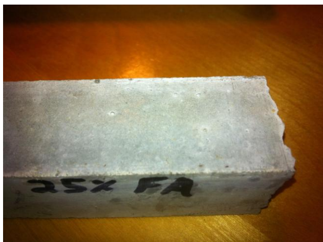
Figure 18: 25FA Mortar Bar. No Signs of Expansion. Figure 19: 10SF Mortar Bar. No Signs of Expansion.
